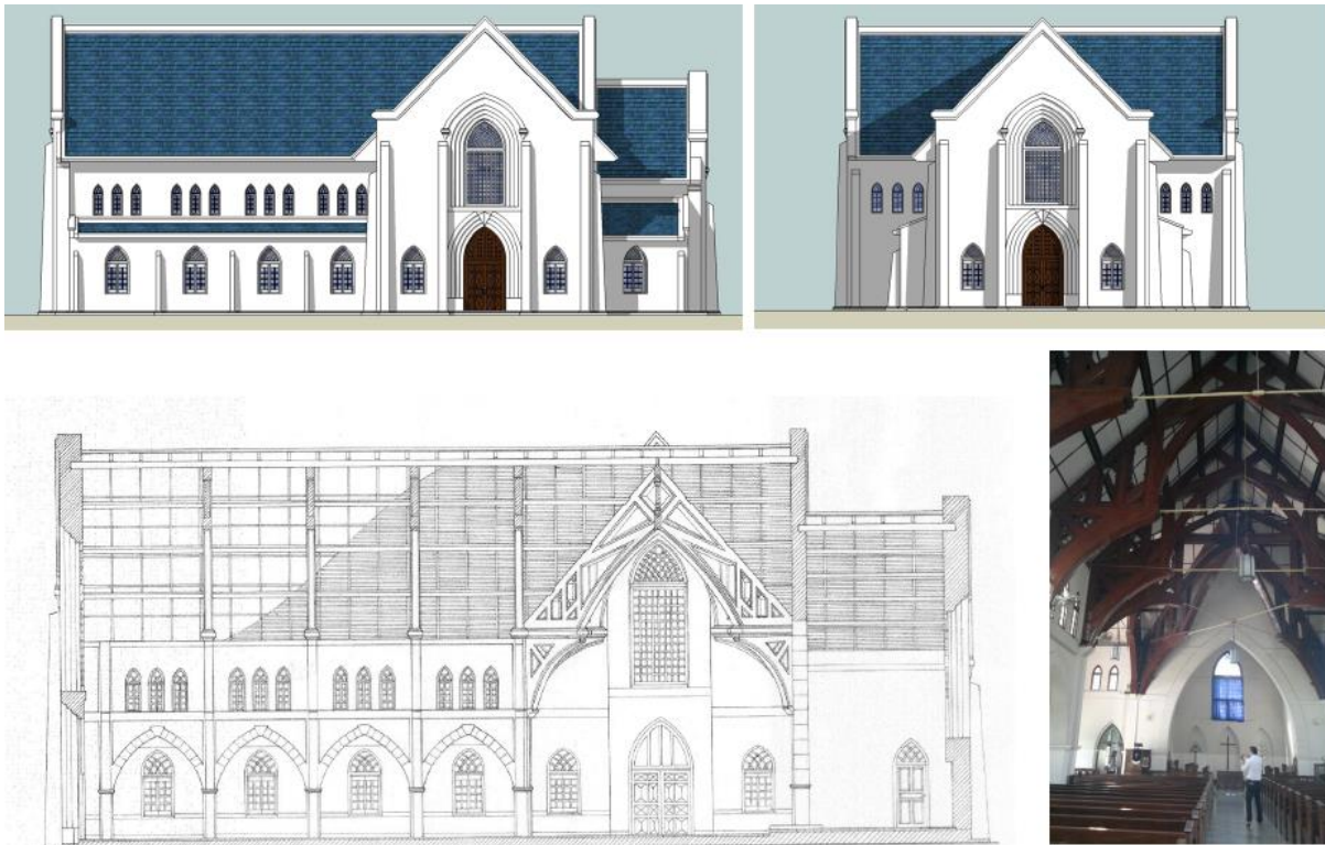
Figure 5: Prince Royal Chapel, built in 1929 by Mr. Van Alan Harris. Adopted the Pitch Roof from Gothic Architecture and re-applied to this chapel using Hammer Beam Roof. Also awarded in 1996 by ASA (The Association of Siamese Architects) to be a well-preserved architecture. [photos by permission of Lanna Architectural Center and Sant Suwatcharapinun]
